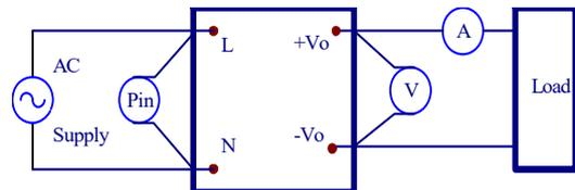
Figure 1. CFM06S Series Test Setup
