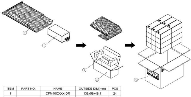
G64F00006 185x155x65 24 2 Antistatic Bag 3 G64301086 Antistatic Foam 155x64x32 24 G64205307 164x73x65 Inner Box 24 5 G64100355 No.78 Cardboard Box 345.4x239.4x284.8
