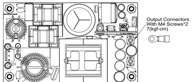
Please allow 4mm side clearance from the components and all side of the PCB. Allow 5mm clearance above the highest parts on the PCB. Be especially careful to allow 5mm between the solder side of the PCB and the mounting surface. If the clearances are not sufficient the specifications for isolation and withstand will not be valid.
