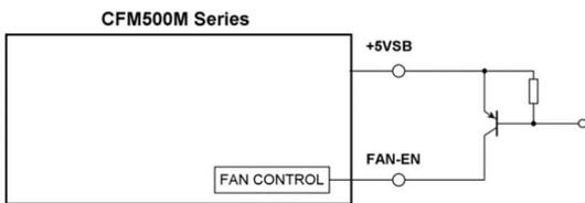
When the PS-On remote control function is not used, connect a short circuit between the pin PS-ON and FAN-EN.
