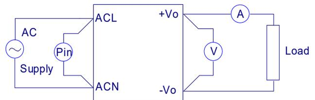
Figure 1. CFM500S Series Test Setup
