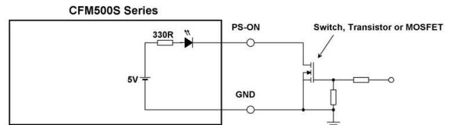
The fan control of CFM500SXXX is provided in CN3 pin 3.
