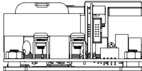
The PS-ON remote control of CFM500SXXX is provided in CN3 pin 4.
