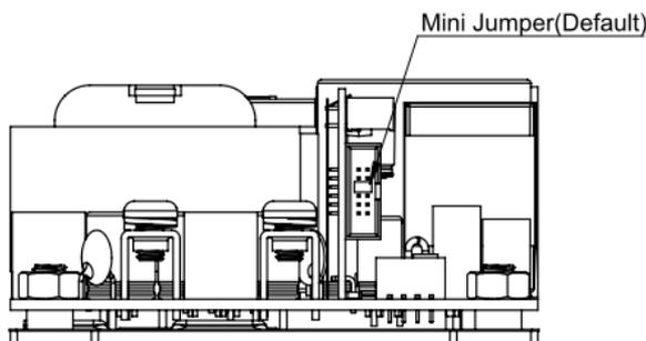
When using the PS-ON remote control and PMBus remote on/off function of CFM500SXXX-PM, remove the Mini Jumper on PS-ON and GND.
