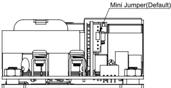
When using the PS-ON remote control and Fan Control function of CFM500SXXX, remove the Mini Jumper on PS-ON and FAN-EN.
