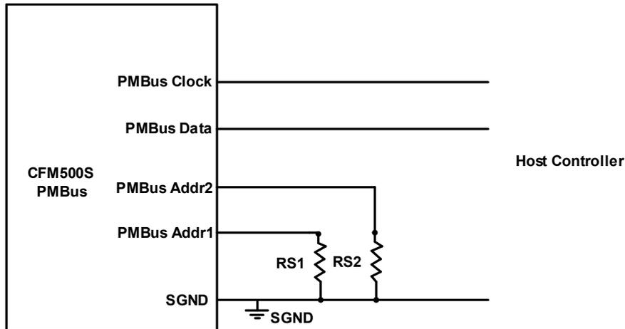
The address for the PMBus is set using external resistors connected to the Addr pins. The table below lists the resistor values for each PMBus address.
