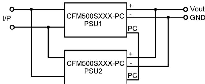
Connect the Pin4 (PS-ON) of CN3 of all PSUs to operate in parallel and start / stop at the same time.
