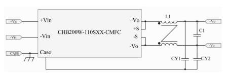
Connection circuit for EMI testing
