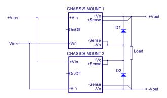
**Simple Series Operation Connect Circuit**
