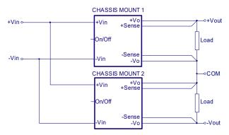
Simple ±Output Operation Connect Circuit
