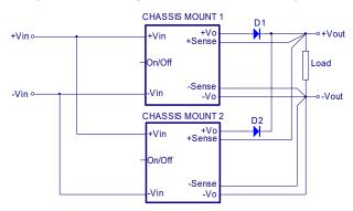
**Simple Redundant Operation Connect Circuit**
