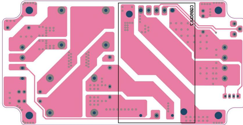
Figure3 PCB layout bottom view
