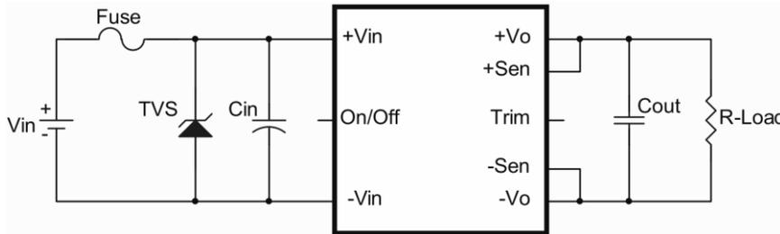
The external input capacitor (Cin) and transient voltage suppressor diode (TVS) are required if CQB50W12 series has to meet EN61000-4-4, EN61000-4-5.
