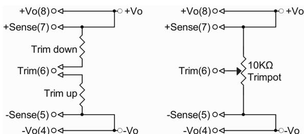
In order to trim the voltage up or down, one needs to connect the trim resistor either between the trim pin and -Sense for trim-up or between trim pin and +Sense for trim-down. The output voltage trim range is -20% to +10%. This is shown:
