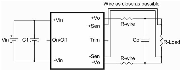
If the remote sense feature is not to be used, the sense pins should be connected locally. The +Sense pin should be connected to the +Vout pin at the module and the -Sense pin should be connected to the -Vout pin at the module. Wire between +Sense and +Vout and between -Sense and -Vout as short as possible. Loop wiring should be avoided. The converter might become unstable by noise coming from poor wiring. This is shown in the schematic below.
