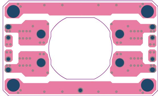
Figure6 Output Filter PCB layout bottom view
