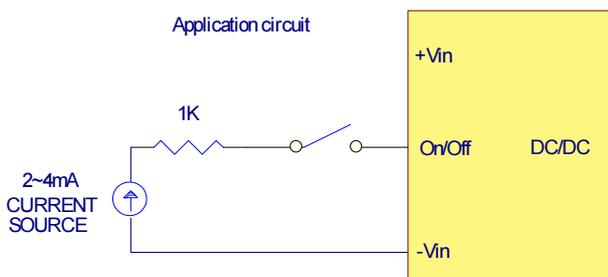
Figure 3 Recommended Application Circuit
