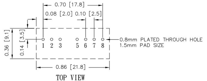
Note: Dimensions are in inches (millimeters)
