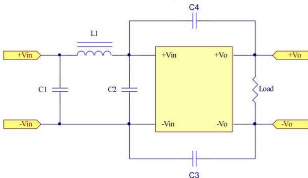
Figure 10 Connection circuit for conducted EMI testing
