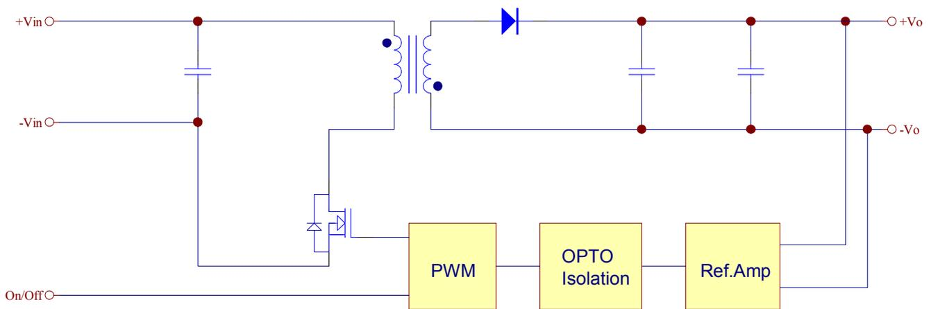
Figure 1 Electrical Block Diagram of single output module
