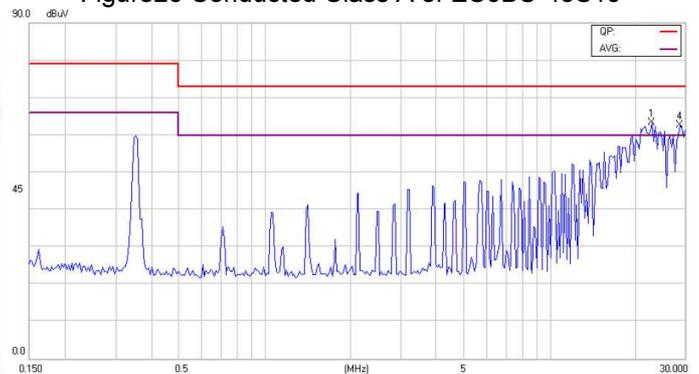
Figure28 Conducted Class A of EC5BU-48D12
