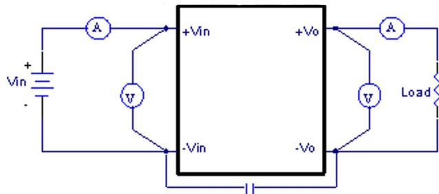
Figure 7 EC5SAW Series Test Setup
