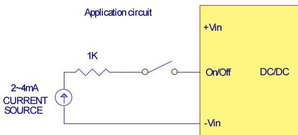
Figure 3 Recommended Application Circuit
