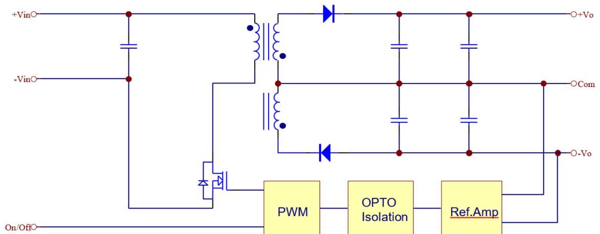
Figure2 Electrical Block Diagram of dual output module
