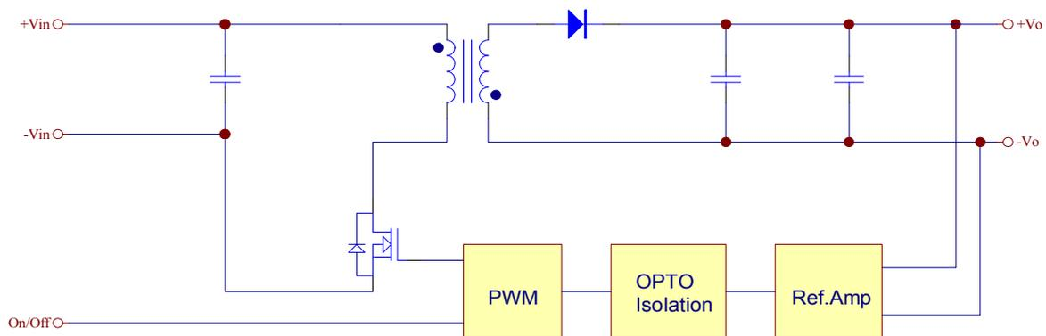
Figure1 Electrical Block Diagram of single output module
