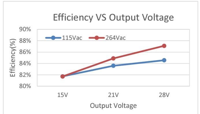
Figure 5 Efficiency vs. Output Power of LDL25 (to Output Current =900mA)
