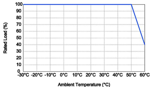
Figure 2. Typical Output power of LDL25 Series
