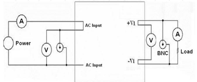
Figure 11. Output Voltage Ripple and Noise Measurement Set-Up
