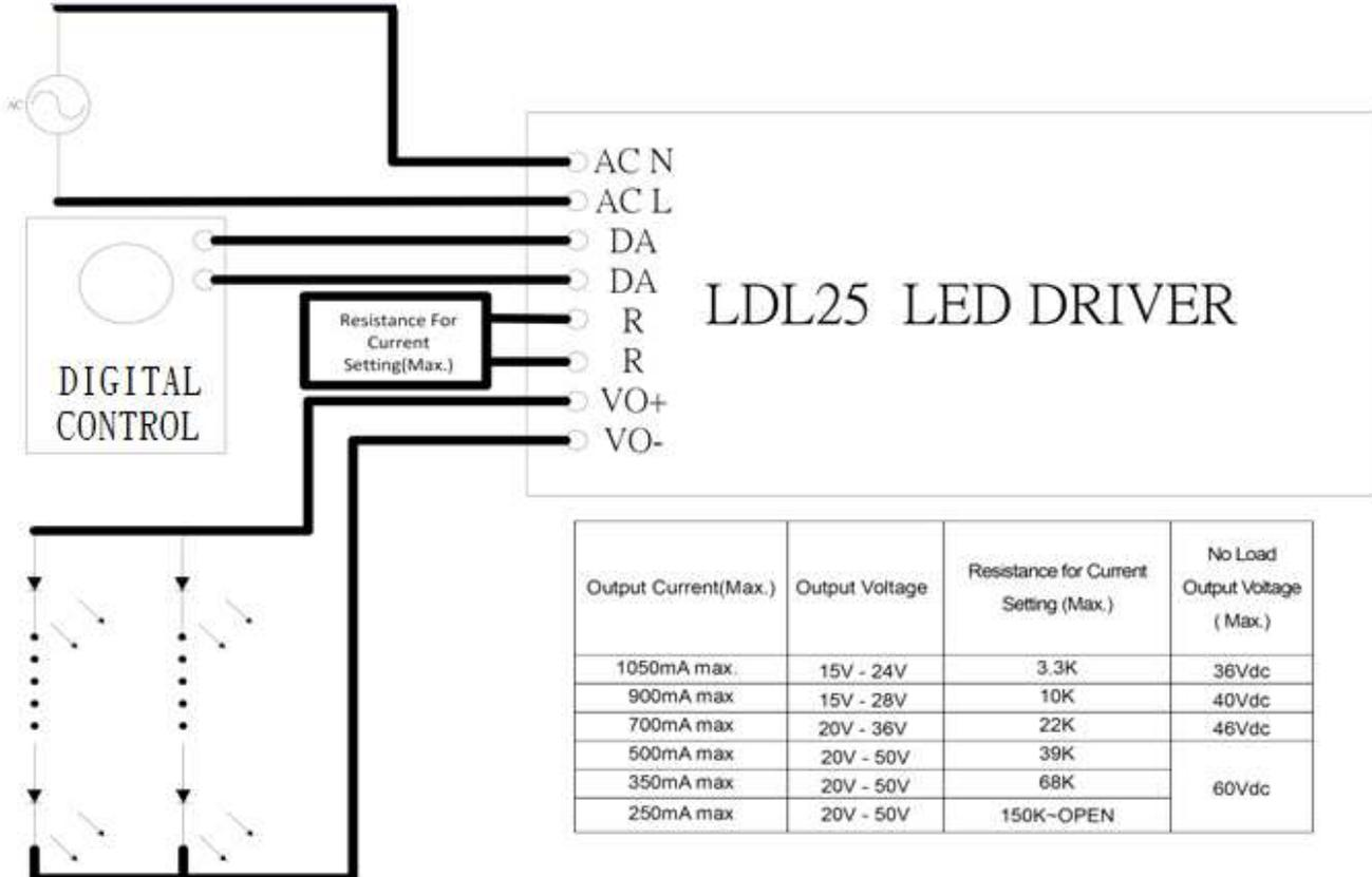
Figure 13 DIGITAL Dimming Function
