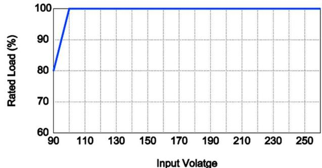
Figure 3. Typical Output Power De-rating of LDL25 (to AC input)
