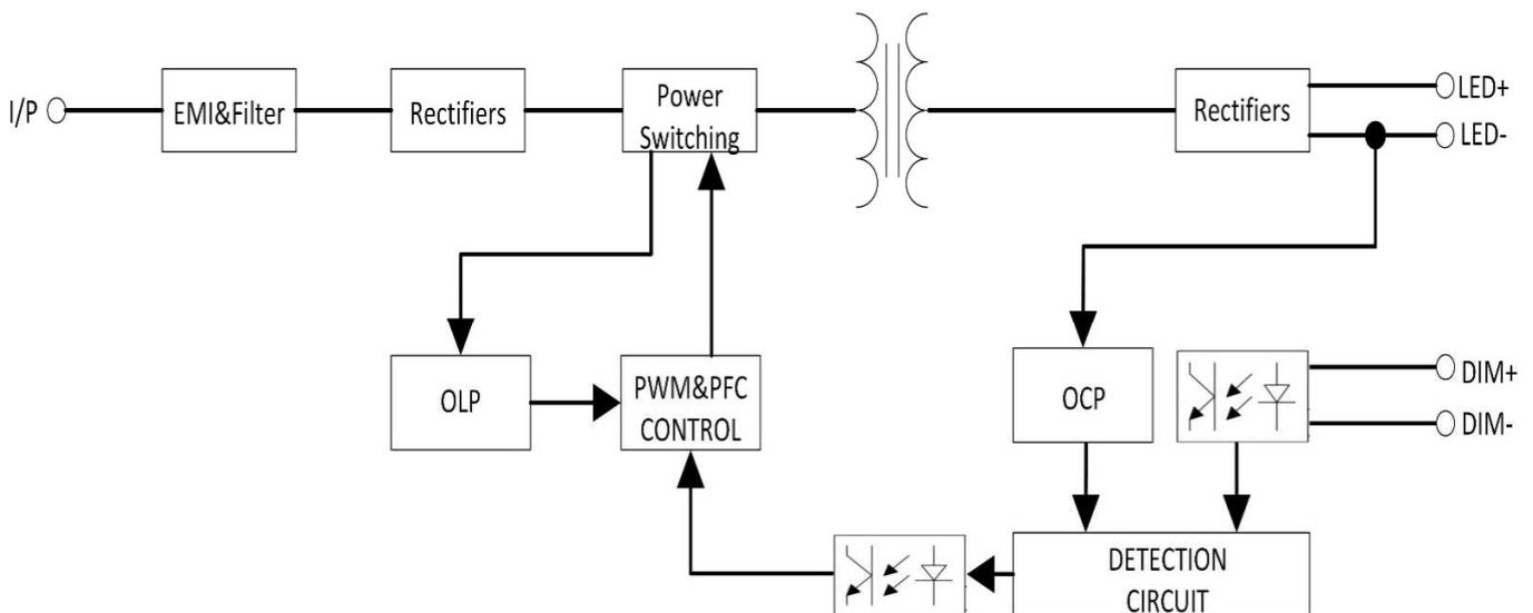
Figure 1. Electrical Block Diagram
