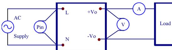
Figure 10. LDL25 Series Test Setup
