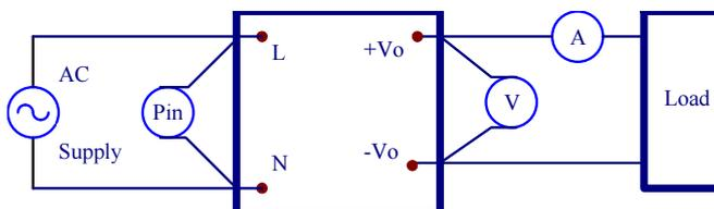
Figure 3. LDM60S Series Test Setup
