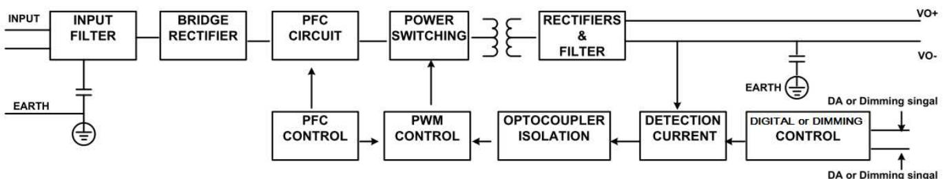
Figure 1. Electrical Block Diagram
