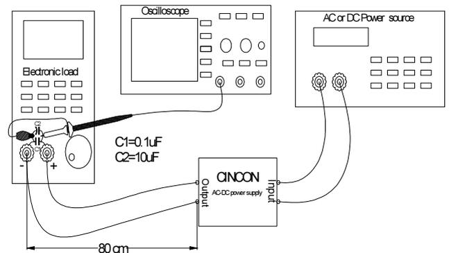
Figure 4. Output Voltage Ripple and Noise Measurement Set-Up
