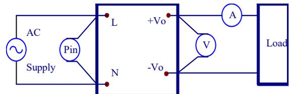
Figure 1. TRE15 Series Test Setup
