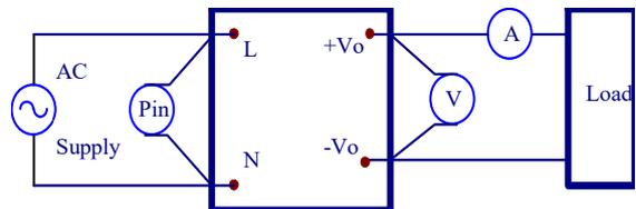
Figure 1. TRE15R Series Test Setup
