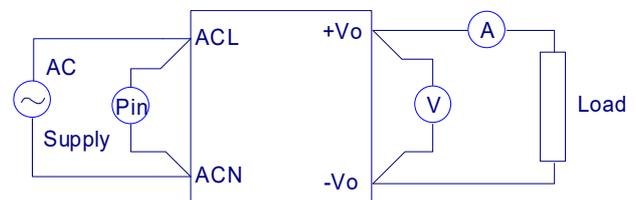
Figure 1. TRE25 Series Test Setup
